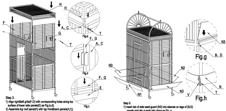
Insert tab of side seed guard (N3) into sleeves on legs of (B,D) panels and slip guards into place as Fig. g.
